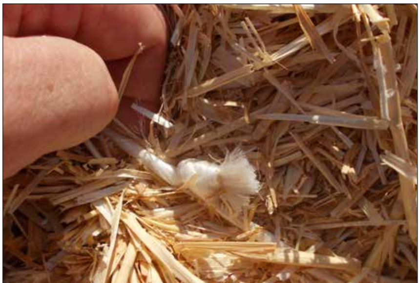
If twine is made only thicker, in an attempt to make it stronger, it may have difficulty holding together as the bale is being formed – so pulling the tail of the knot through and risking the knot coming undone.
