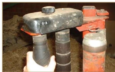
Check that gear box is not damaged
