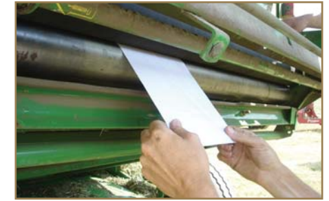
an easy check for feed roller setting can be done with a sheet of paper
