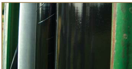
Remove any tack build up on pre-stretch rollers with solvent based cleaner
