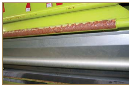
rusty net roll brake bar will damage net
