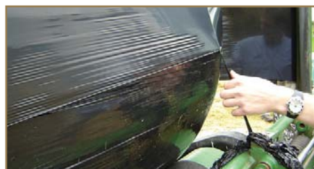
if film is not released at start of wrap cycle it will allow air into the bale.
