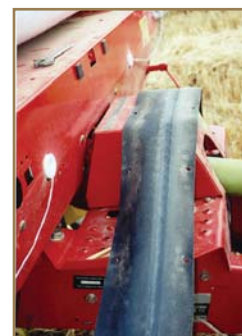
worn rubber strip on brake bar will reduce braking action against net roll
